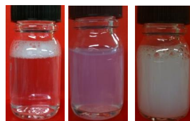
Figure 14 -Polymerization sample of FREPE ([1] -1h, 100 bar); ([2] -2h, 200 bar); ([3] -8h, 200 bar) (50 mg AIBA, 0.3 g PEG-X, 250 rpm, T=70^{\circ}\text{C} ).
